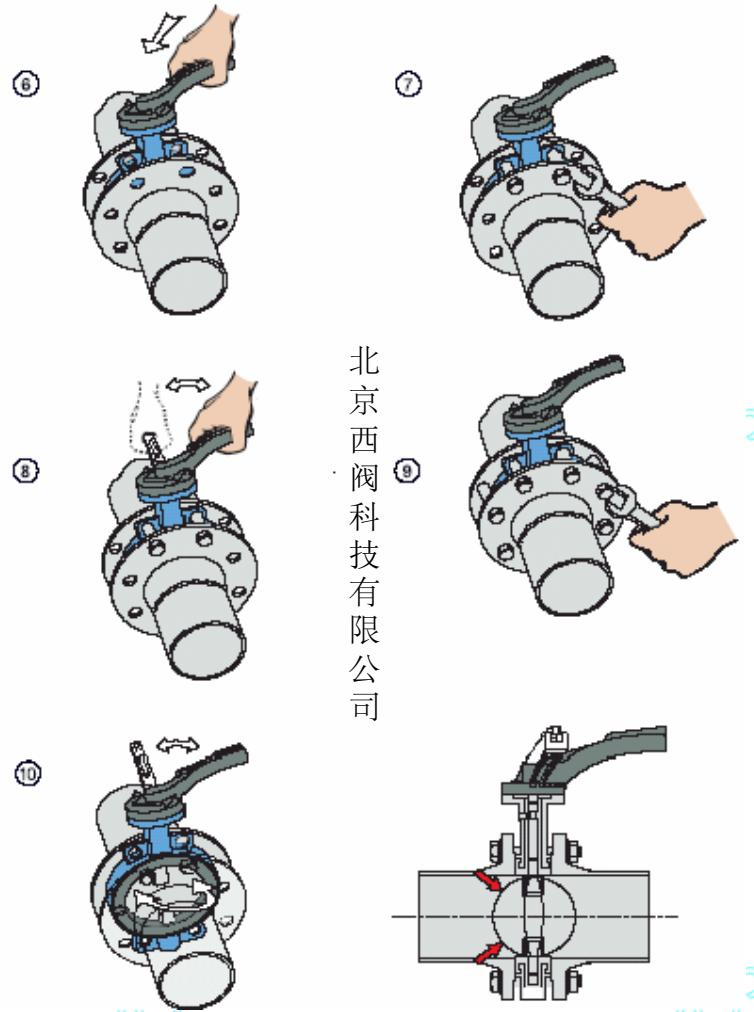
⑥ Let flanges cool down and re-install the valve. The valve must move easily between the flanges to prevent damage to the collar. Leave valve disc slightly open.
